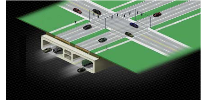
3 Cut-and-cover tunnel below rebuilt Highway 3/Huron Church Road Corridor.
